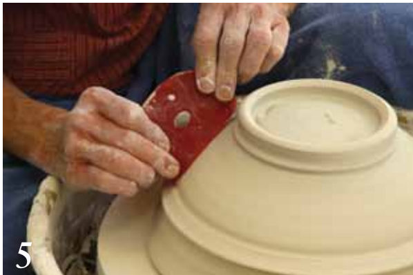
5 Refining and smoothing the trimmed surface using a rubber rib to remove any lines or marks.
