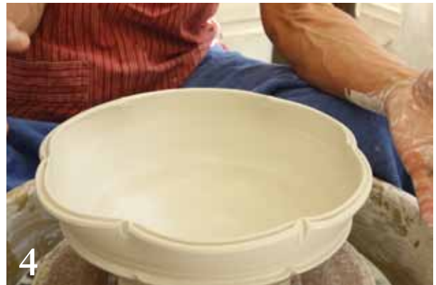
4 Divide the rim of the bowl using a circle divider and marking tool. Press in at each mark, creating six lobes.
