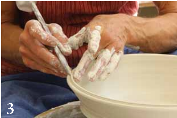
3 Refine the split rim using a wooden knife or rib while supporting the rim on both sides as you work.
