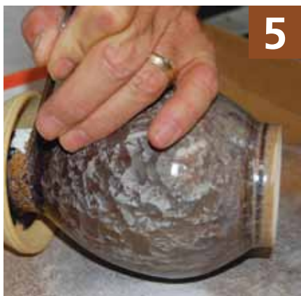
The pedestal and catch basin are removed by tapping with a small chisel along the line where the pedestal joins the pot.
