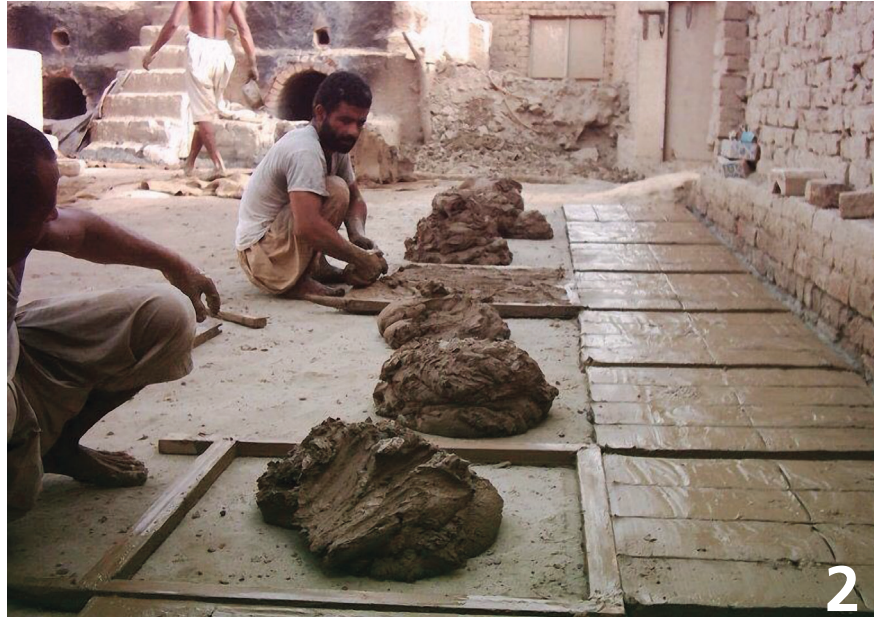
1 The clay used to make kashi tiles is brought from the river basin. The tile makers screen the clay, then mix it with water. 2 Next, they lay it out in wooden molds to dry to a usable consistency prior to cutting into smaller slab shapes using a wooden frame (called a karab).
