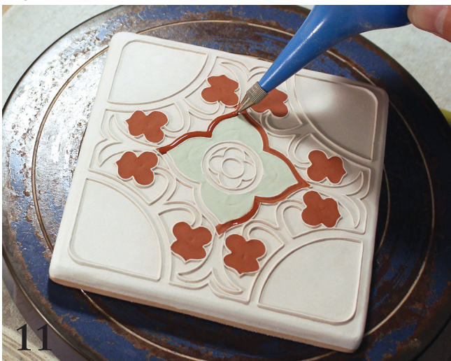
11 Spray water on the bisque-fired tile so the glaze flows evenly, then use a filled bulb syringe to glaze in between the raised lines.
