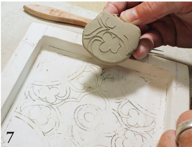
7 Once an area has been initially carved, check the pattern by pressing a slug of clay into the mold then lifting it out.
