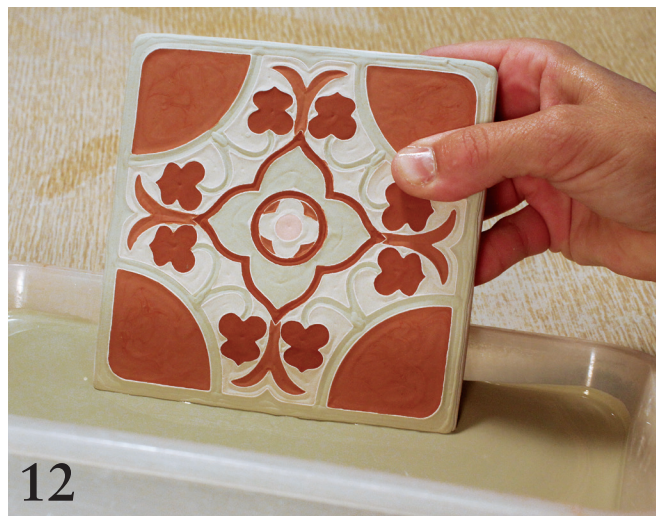
12 Once the bulb-syringe-applied glazes are fully dry, dip the edges on all sides in a tray of glaze prior to the final glaze firing.
