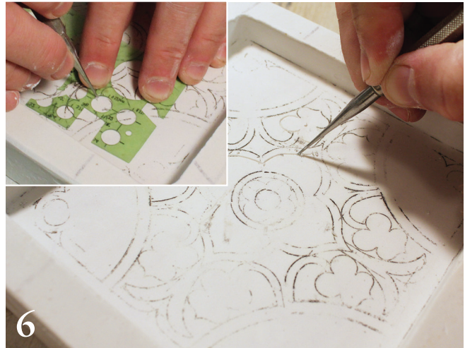
6 Carve the tile with plastic templates and dental tools after the plaster has set but before it completely dries out.
