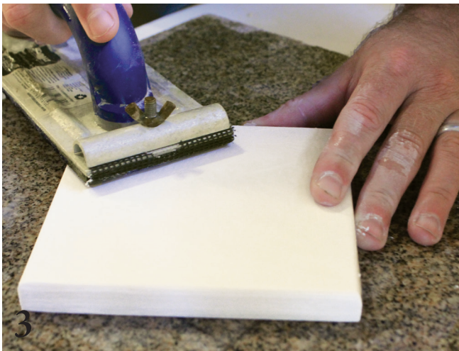
3 Sanding the square plaster tile master with drywall sandpaper before switching to finer grits of wet/dry sandpaper.
