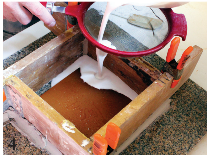
4 Pouring the plaster negative cavity from the master rubber positive that was created first.
