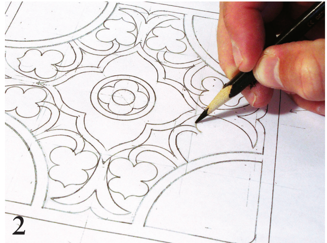
2 Drafting the Flores tile using both plastic templates and freehand drawing.
