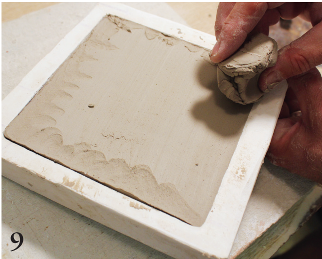
9 Fill in the rest of the mold with clay, scrape away excess clay, level the tile, then remove the tile with a slug of clay.
