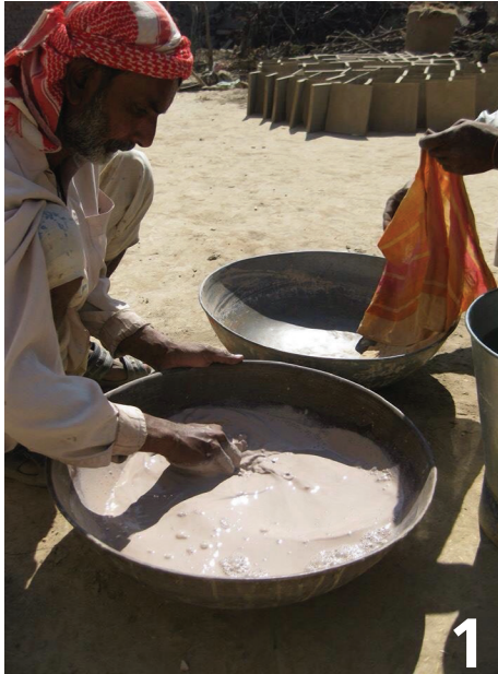
1 The clay used to make kashi tiles is brought from the river basin. The tile makers screen the clay, then mix it with water. 2 Next, they lay it out in wooden molds to dry to a usable consistency prior to cutting into smaller slab shapes using a wooden frame (called a karab).
