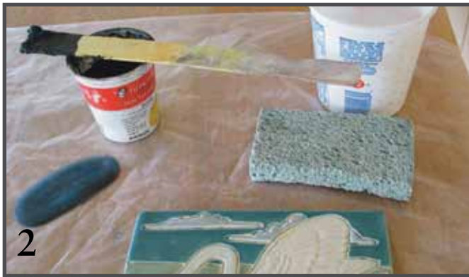
2 Necessary tools: plastic drop cloth, gloves, containers, water, sponge, stir stick, grout, and squeegee.
