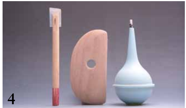
4 Left to right: A disposable paint brush handle with the plastic support trimmed down, a wooden rib, and a squeeze bulb with a piece of an ink tube and a guitar string.
