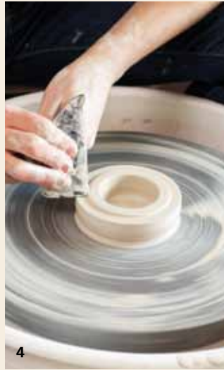
4 Throwing the lid's flange with a wooden rib.
