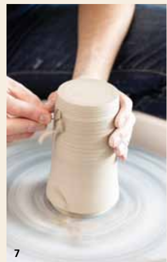
7 Trim the exterior wall of the leather-hard jar using a ribbon trimming tool.
