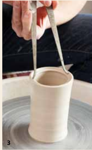
3 Measuring the width of the jar's gallery with calipers.
