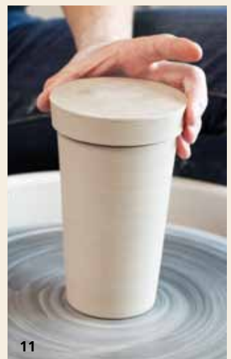
11 Place the lid onto the jar and assess the fit of the rims and of the lid flange.
