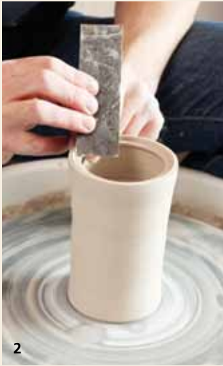
2 Throwing the gallery with a steel rib.
