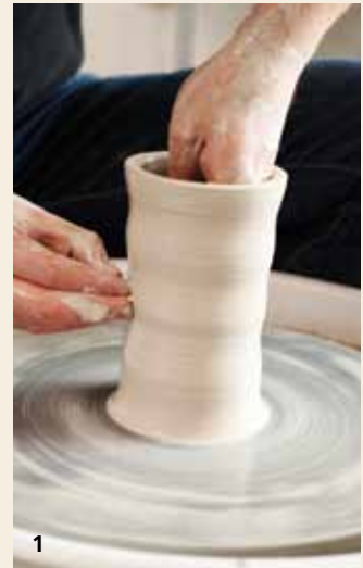
1 Throwing the jar. An appropriate height is usually achieved in three pulls.
