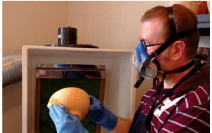
Nichols uses a respirator and a hooded exhaust vent to manage the dust created when sanding his dry surfaces. Below is a surface detail revealing the layers of colors.
