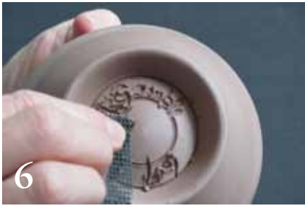
6 Remove burrs using a damp sponge or drywall sanding screen before the bisque firing.
