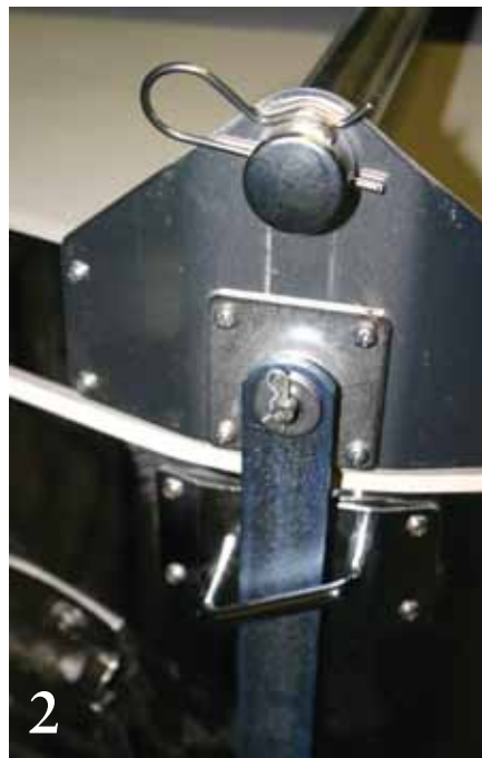
2 Inspect hinges and lid handles for wear. Tighten loose screws or pins.
