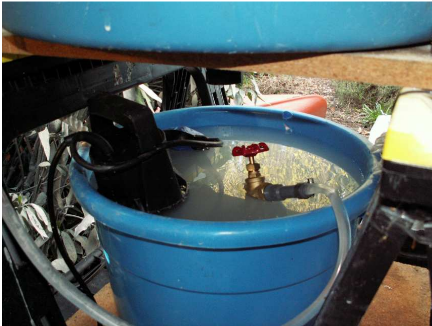
Sump pump (6) and hose to feed water to the sprayer. Valve to control flow (7). The sprayer sits on two plastic sawhorse's (6)
