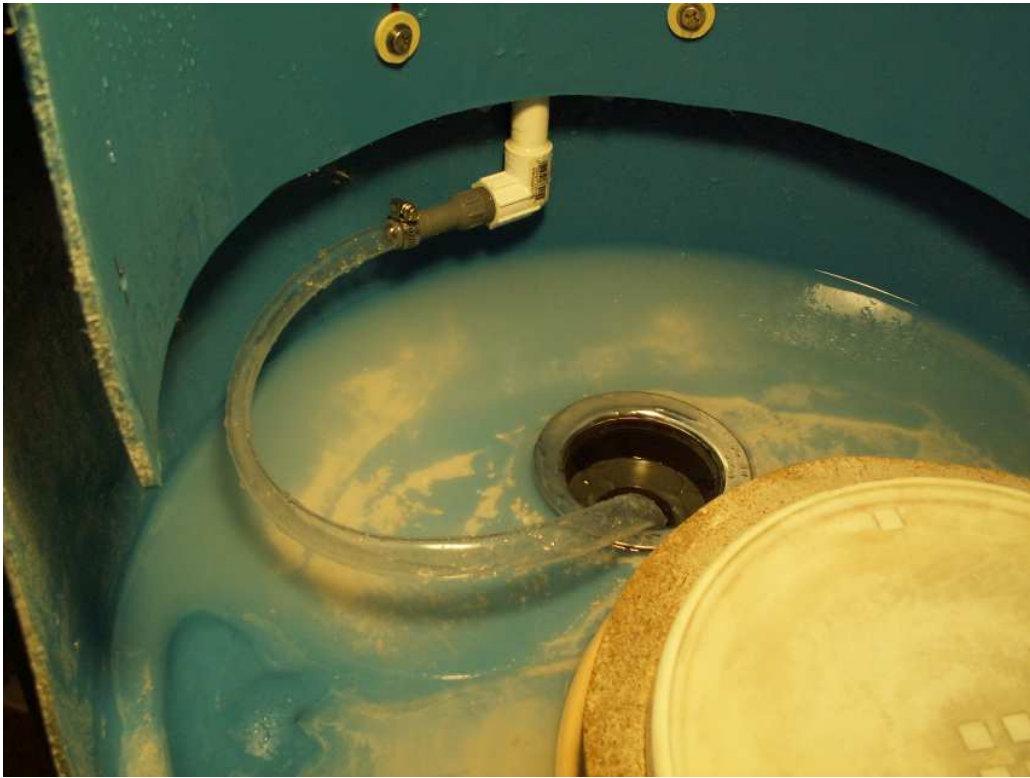
Water connection from pump to pipe to sprayer. I routed the pipe up through the middle of the drain.
