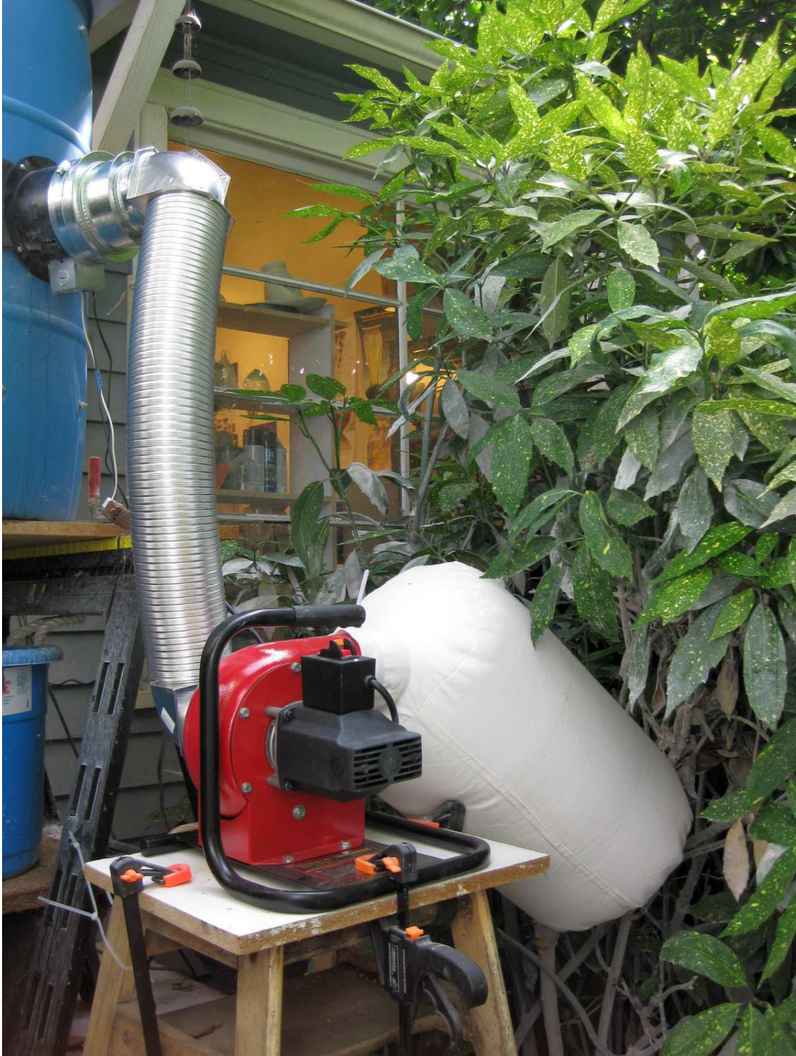
Stronger exhaust system and filter (9) with dryer vent pipe and fittings (10)
