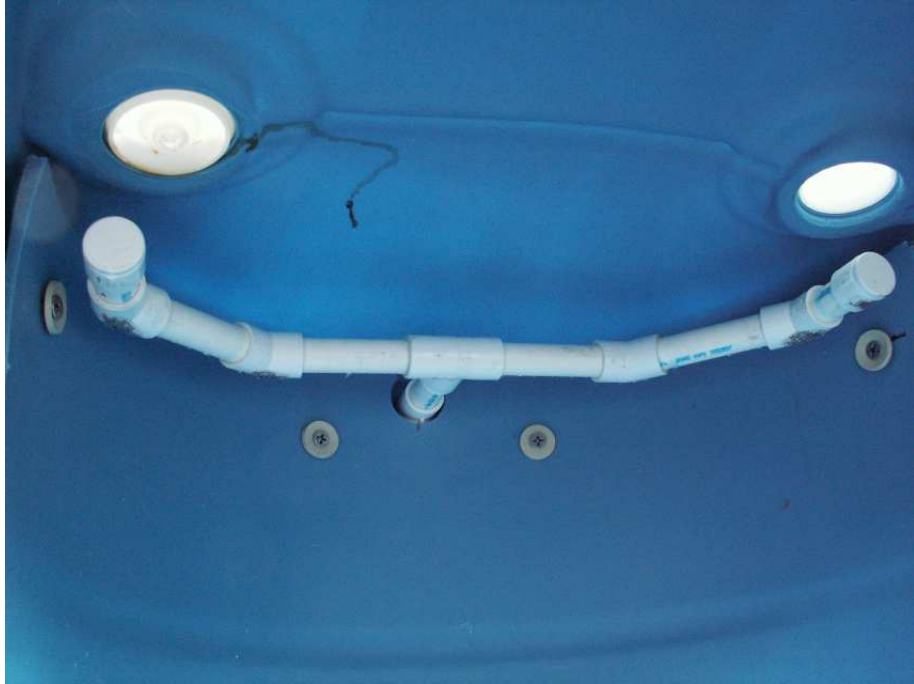
This sprayer (version 1) is made of 1/2" pipe and 45° connectors. Small holes are drilled along the backside (see detail next)
