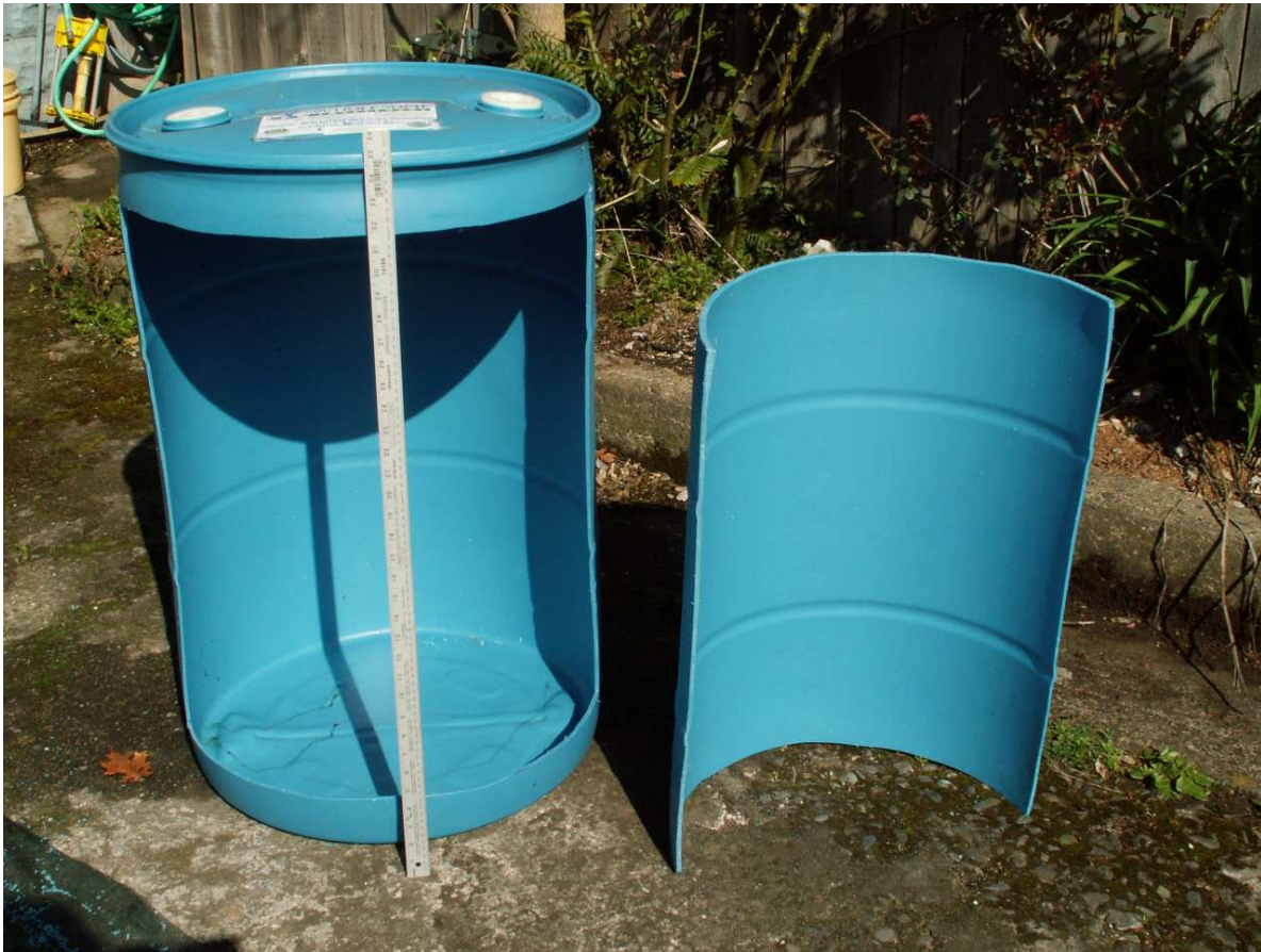
I drilled four holes at the corners of the cutout then I cut it out with a jig saw. I left 3 inches on the top and bottom. The opening is about 22" w by 28" h.
