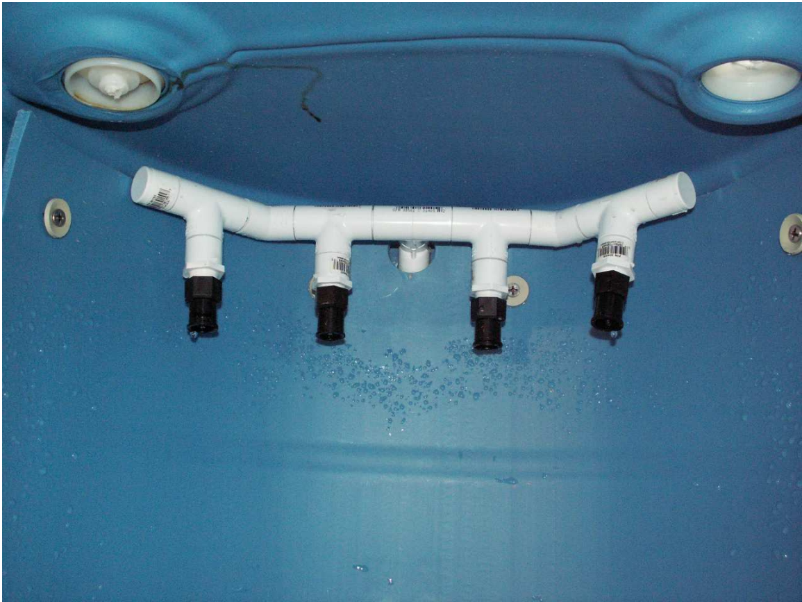
Sprayer assembly version 2. This uses sprinkler heads to disperse the water.
