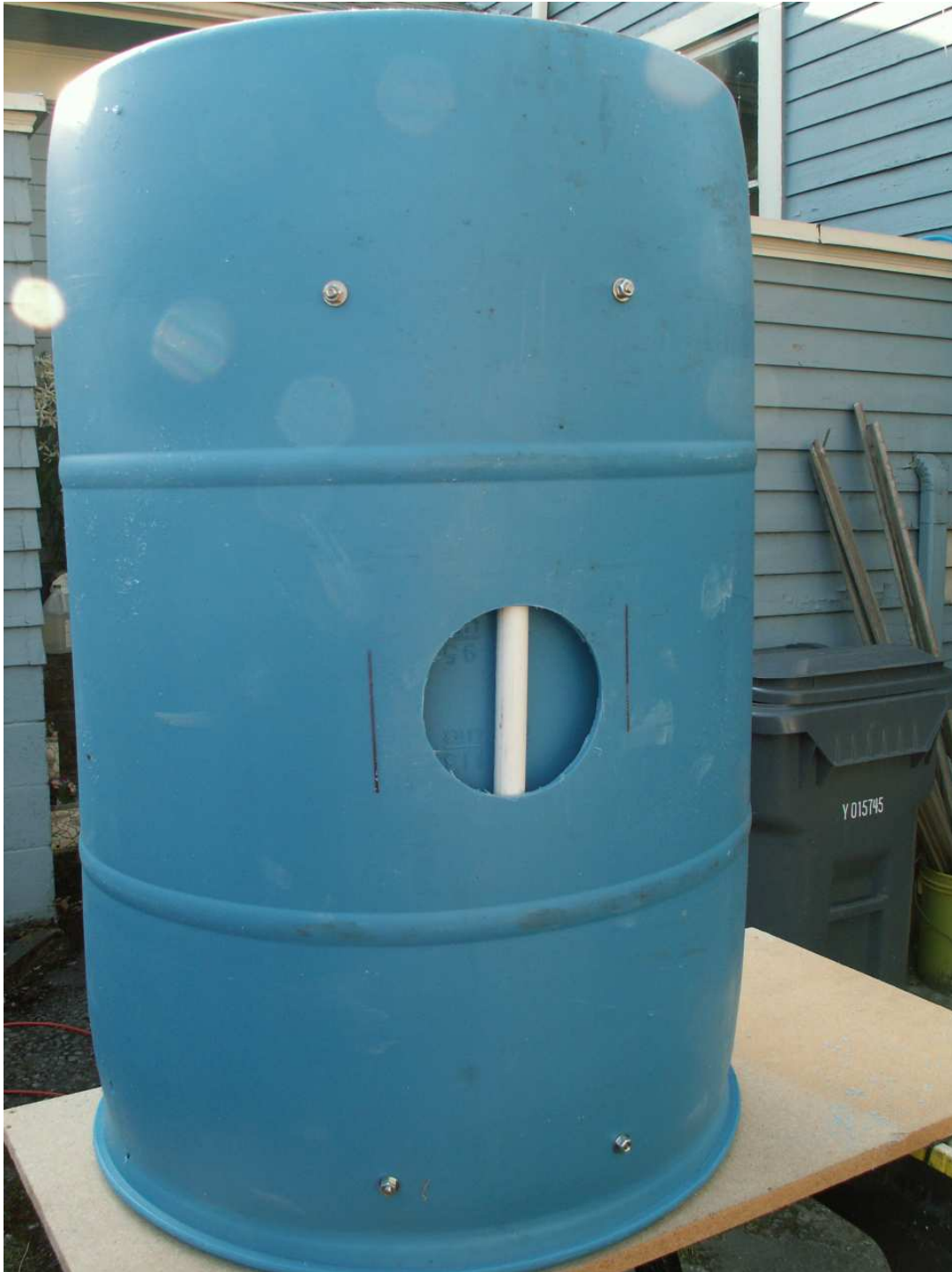
4 1/2 inch hole in the back wall for the exhaust fan. I had to push the pipe out of the way before I drilled the hole. This will pull air through the booth. Eventually there will be a structure to hold a filter. But for now.....
