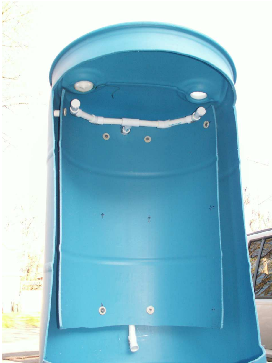
Sprayer in place.
