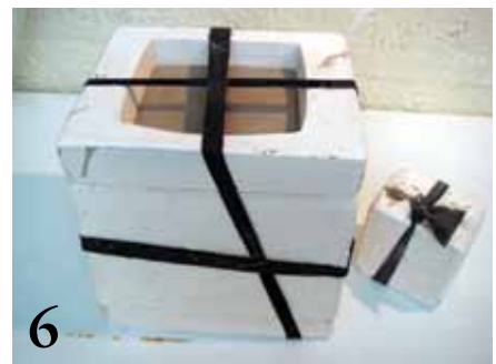
6 Secure separate parts of a plaster mold before filling with casting slip.
