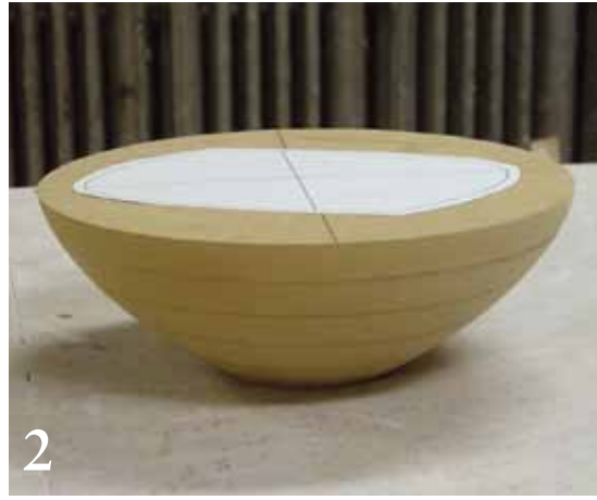
2 Turn a solid, laminated MDF form on a lathe to get close to the right profile.
