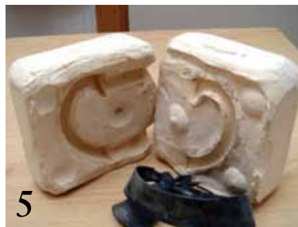
5 Plaster mold for the handle. The two openings allow air to escape.
