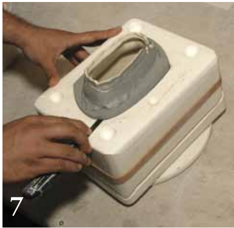
7 Cut away the pouring gate. Keep the blade flat on the top of the mold.
