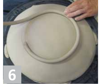
6 Center the mold on the wheel, make marks for the foot ring and extrude a ½-inch coil for the foot.
