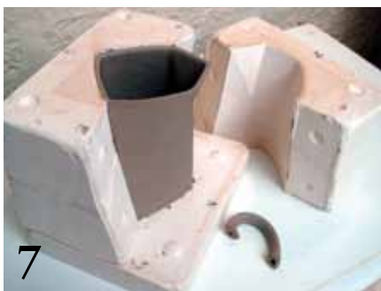
7 Allow the forms to set up before removing them from the molds.
