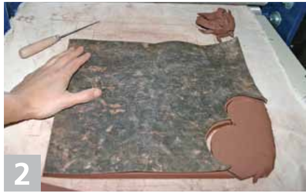
2 Use a tarpaper template to cut a slab for the mold.
