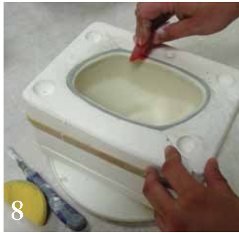
8 Finish the rim with a red rubber rib. Note the striations of contrasting colored slip.
