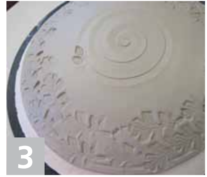
3 Add a throwing spiral with a metal rib and create emphasis with a small leaf stamp. Dry and bisque fire.
