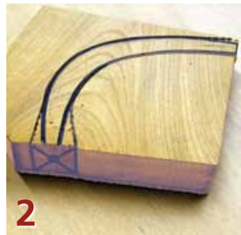
2 Be sure to leave extra wood on each end of the egote to facilitate drilling the holes.
