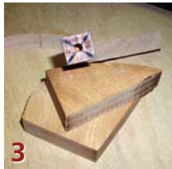
3 Find the center, cut out the curved form and drill ¼-inch diameter holes for the dowel connectors.
