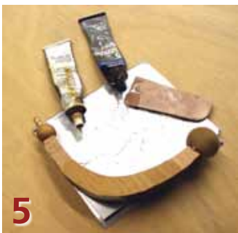
5 Epoxy the dowels into the drilled holes on the stick. Trim off the dowels after the glue dries.
