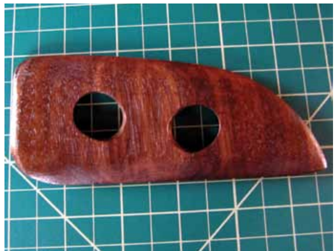
The finished rib with customized curves and finger holes.
