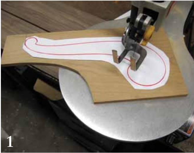
1 Trim and attach the paper using double-sided tape. Cut out the rib leaving the tracing in place.
