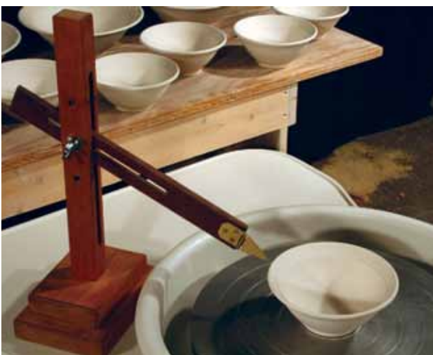
The Fulwood Measure from Kissimmee River Pottery ( www.kissimmeeriverpottery.com ) is an example of a Western pot gauge. When the rim meets the hinged pointer, it folds out of the way.
