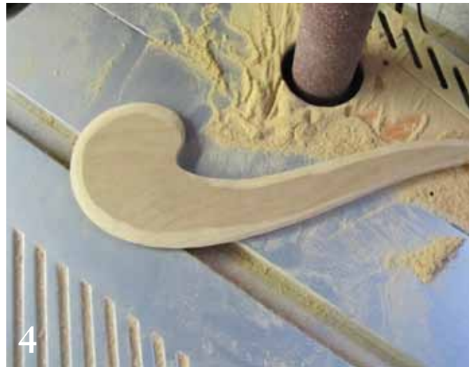
4 Taper the edge of the rib by angling the piece as it is brought to the sander and move with long strokes.
