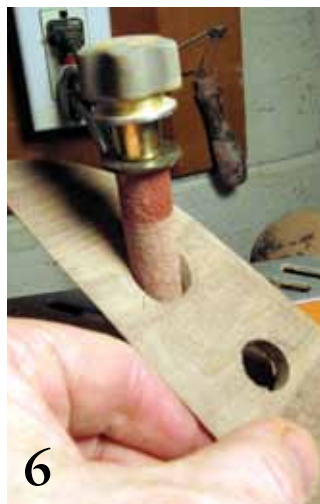
6 Smooth each hole then tilt the rib to mimic the marks made by your fingers.
