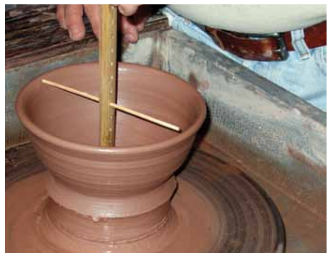
The tombo measures the inside depth and width of a form. Two sources of tombo are Bamboo Tools ( www.bambootools.com ) and Chris Henley (inset) at http://hominid.net/toolpage2.htm .
