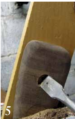
5 Drill \frac{5}{8} -inch finger holes where your fingers naturally grasp.
