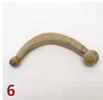
6 Use wood rasps to begin to rough out the final shape.
