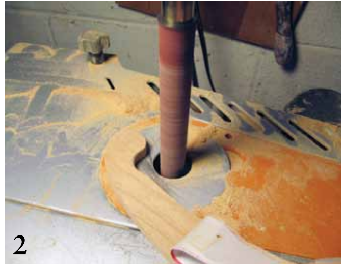
2 Fine tune the finger groove at the small end and customize the overall shape using a spindle sander.
